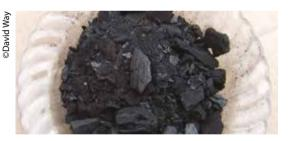
Pure charcoal. A grade composed of small lumps and powder such as this can be referred to as *Biochar*. Its structure is highly microporous and provides an attractive environment for many microbes in the rhizosphere.
